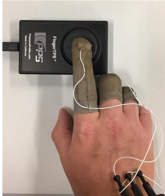
Figure 2.3 – Calibration of FingerTPS sensors using provided load cell.
